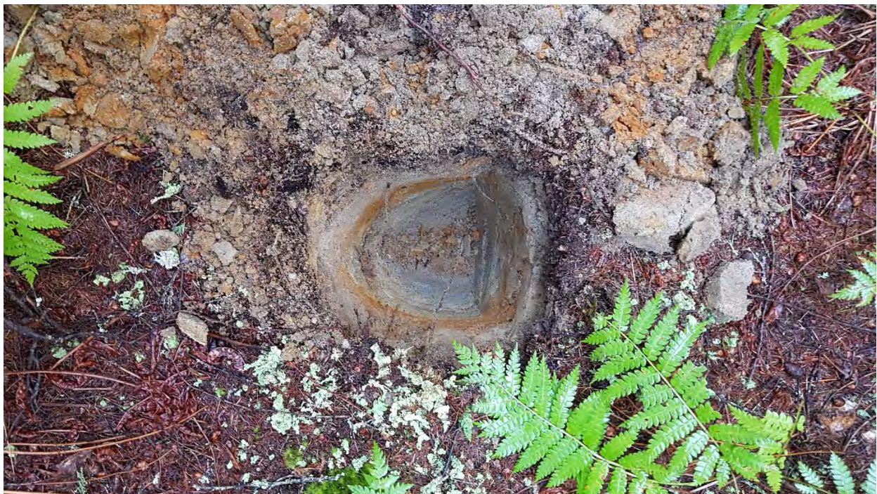
Photo 8. Area 3B – The upland soil is also grey coarse sand, showing signs of leaching and iron accumulation in the upper part.
