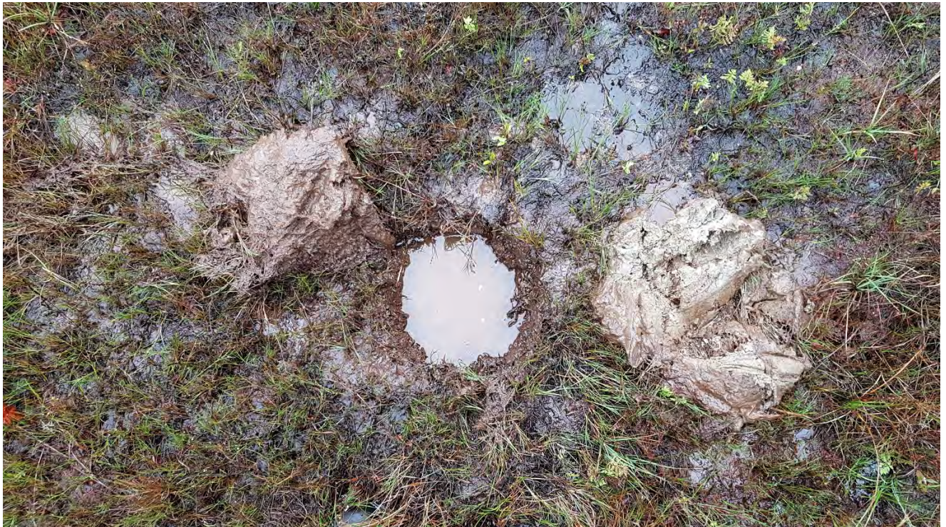
Photo 12. Area 3C – The wetland soil is grey coarse sand, identical to other tailings impacted sites. The sand substrate is dense and firm to walk on.
